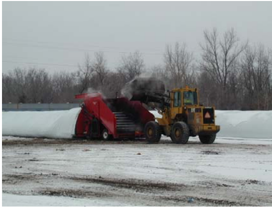
Front loader loading processed compostable waste into in-vessel bags at NRG PS.
