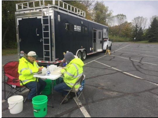
Project partners at the United States Geological Survey arrived with a mobile laboratory to monitor zebra mussel mortality and chemical concentrations during the EarthTec QZ treatment.
