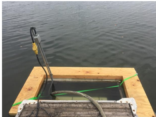
Lake water is continuously tested during the treatment and pumped to tanks on shore with live zebra mussels to measure chemical concentration and zebra mussel mortality.
