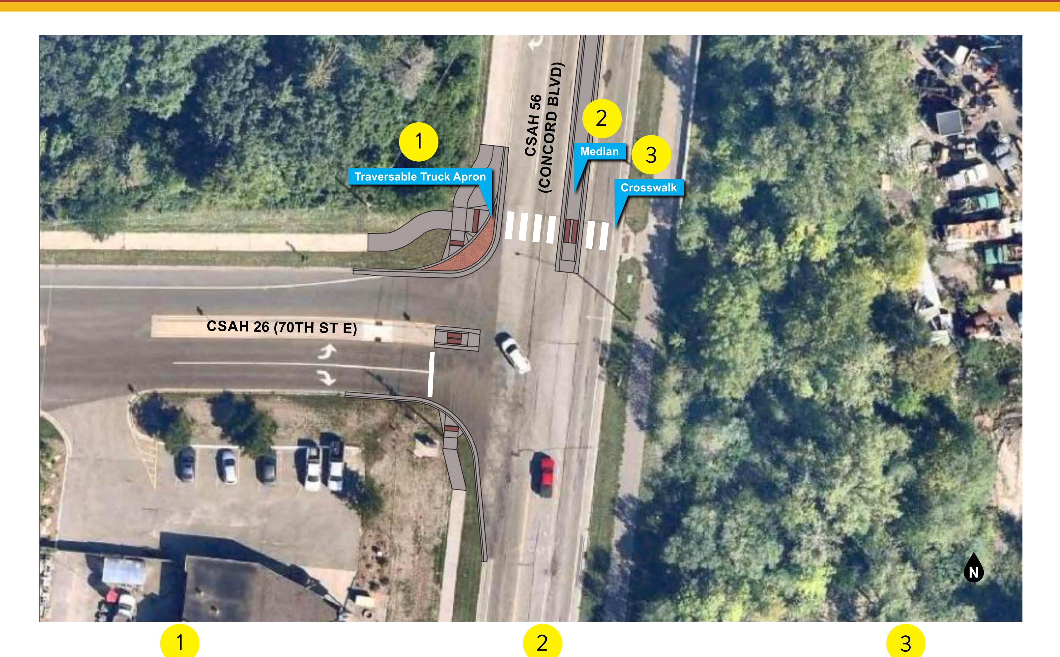
Transversable truck aprons slow turning vehicle speeds, while providing space for large trucks to complete their turns.
