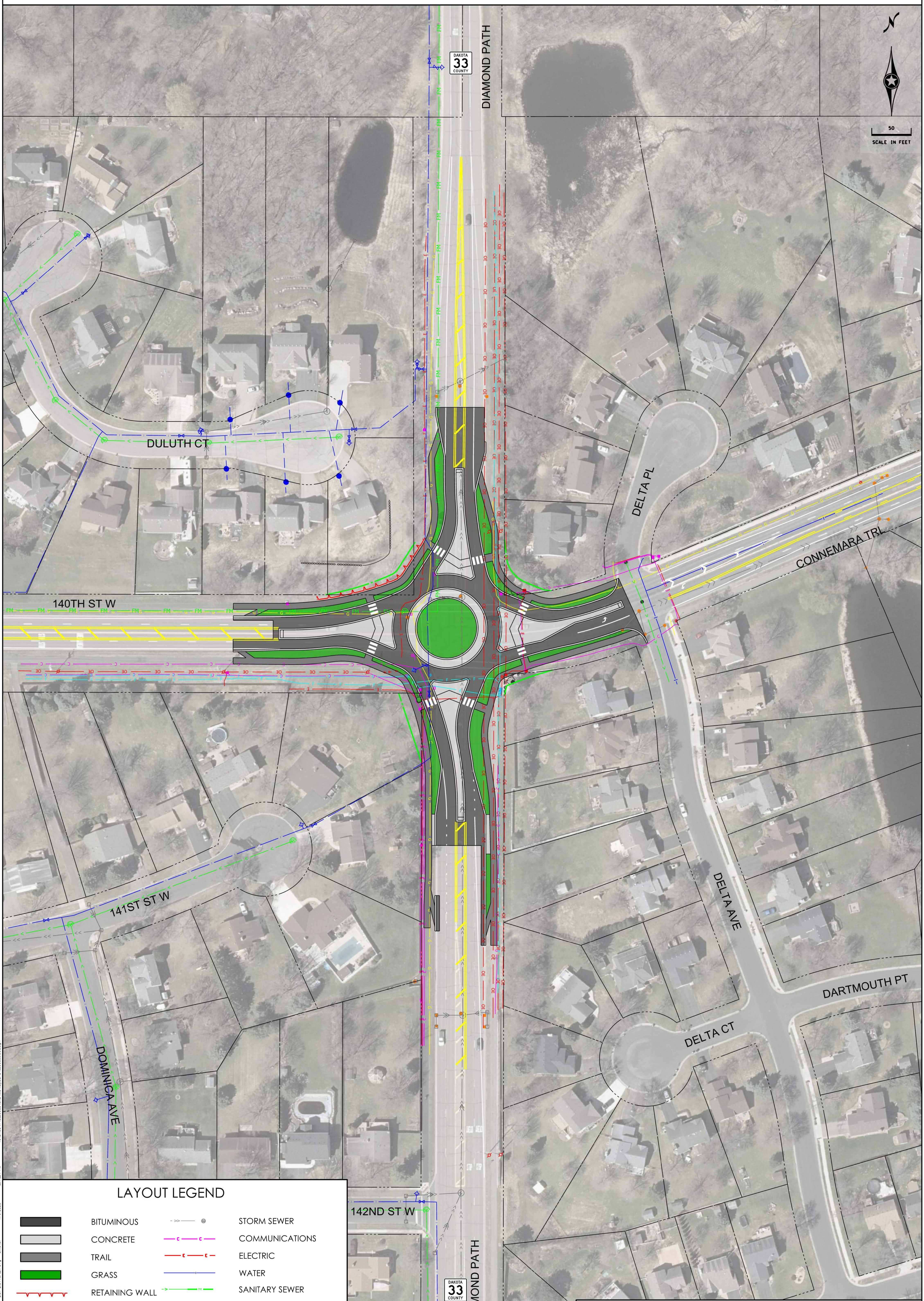
SINGLE-LANE ROUNDABOUT: CONCEPT 2b CSAH 33 (DIAMOND PATH) at 140th STREET/CONNEMARA TRAIL
