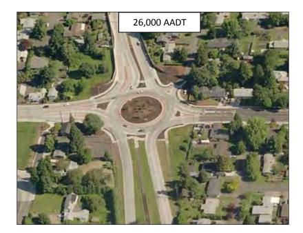
20 Year Projected AADT: 57,000 N-S Speed Limit: 45 mph E-W Speed Limit: 35 mph No yielding problems at entering.
