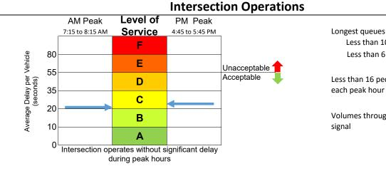
Longest queues are: Less than 10 vehicles for NB & SB Less than 6 vehicles for EB & WB
