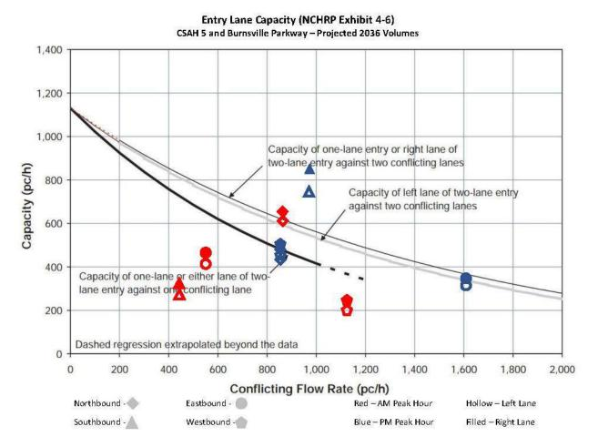
As shown, in the morning peak the traffic for the northbound approach is just above the capacity of the roundabout. In the afternoon peak, traffic on the southbound approach is well above the capacity. The concentration of volume on these approaches means more traffic than expected gaps in traffic, leading to the capacity issues identified.
