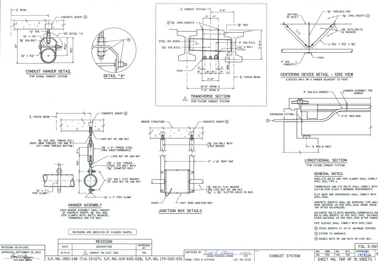
RODS, EYE BOLTS AND PIPE CLAMPS SHALL COMPLY WITH
