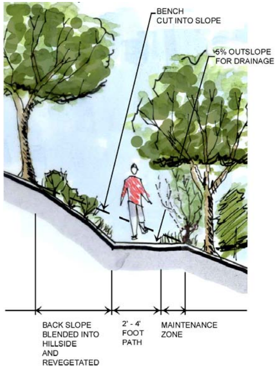
Figure 5.7 - Trail on slope with full bench construction and outslope
