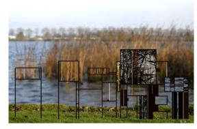
STEEL FRAMES WITH TEXT INSETS Weathered steel finish to match sign blades. Graphic panels to be stud mounted to frame. Base of frame bolted to concrete pad.
