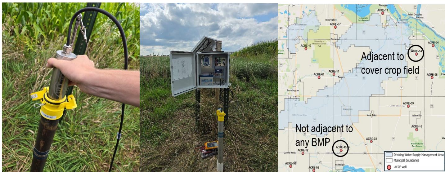
Figure 2. (a) close-up of nitrate probe in well; (b) nitrate sensor set-up; (c) ACRE wells with nitrate probes.
