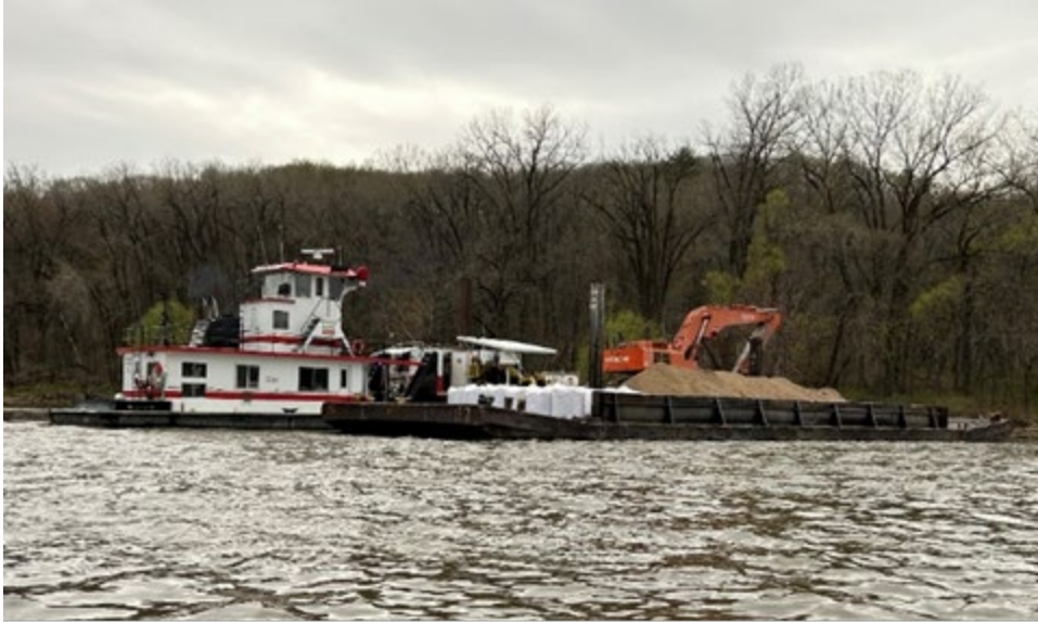
Figure 2. Barge with sand and bags of bentonite used for the well sealing.
