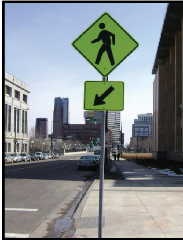
Example of recommended pedestrian crossing sign (W11-2) and down arrow (W16-7P) for a mid-block crosswalk
