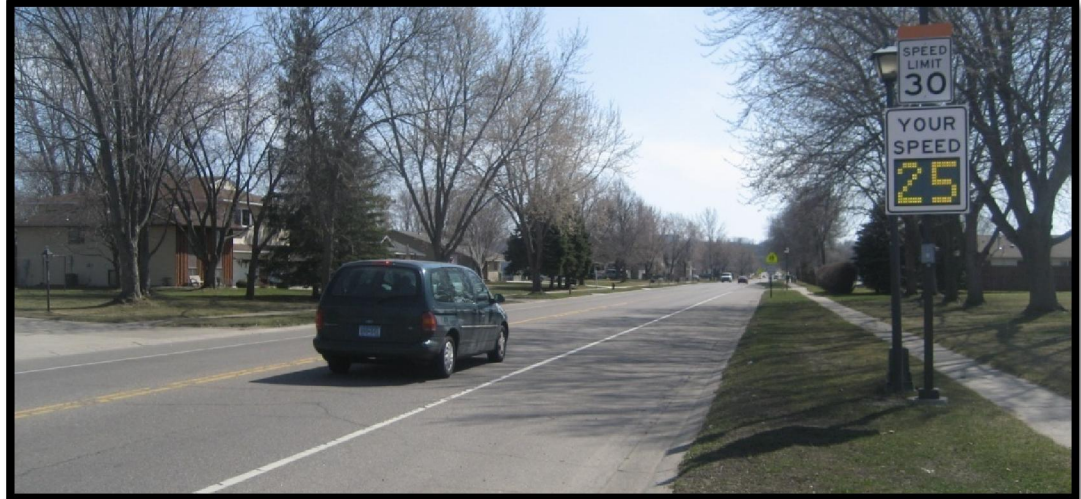
Example of a driver feedback sign that displays the vehicle's speed as well as the posted speed limit.
