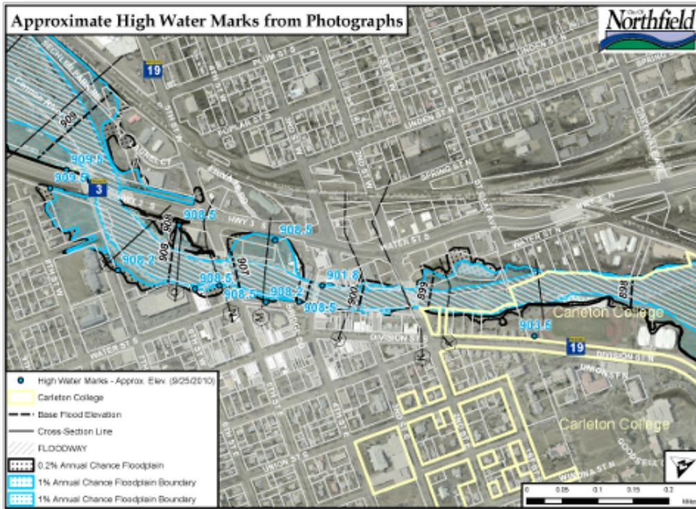
*Figure 4. Map of high-water marks mapped from photographs taken at the crest of the flood, existing high-resolution aerial photos, and LIDAR-based contours. 2003 FEMA flood boundaries are shown for reference.*
