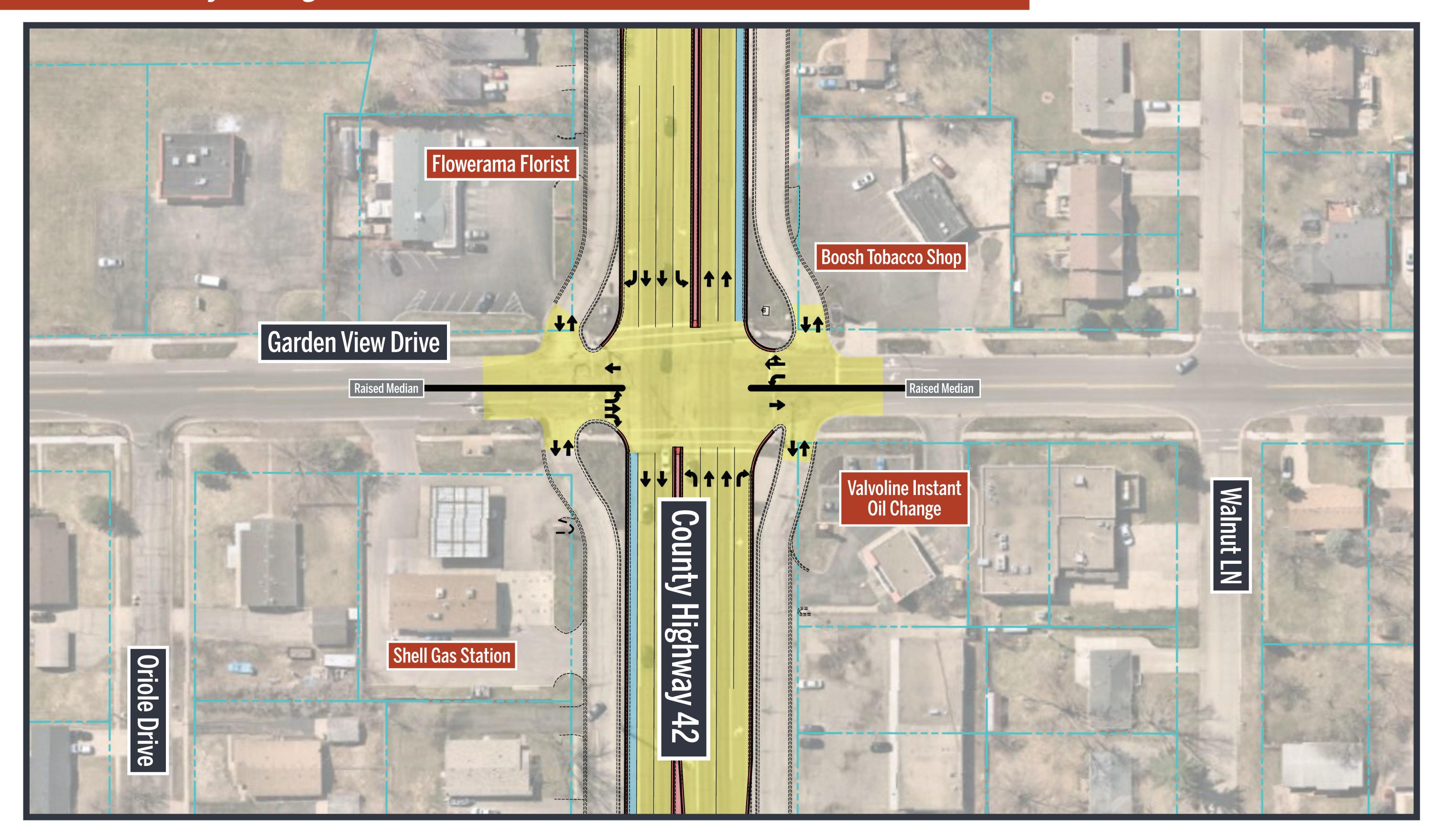
Alternative 4: Two-Way Frontage Roads with Extended Raised Medians and Mini-Roundabouts
