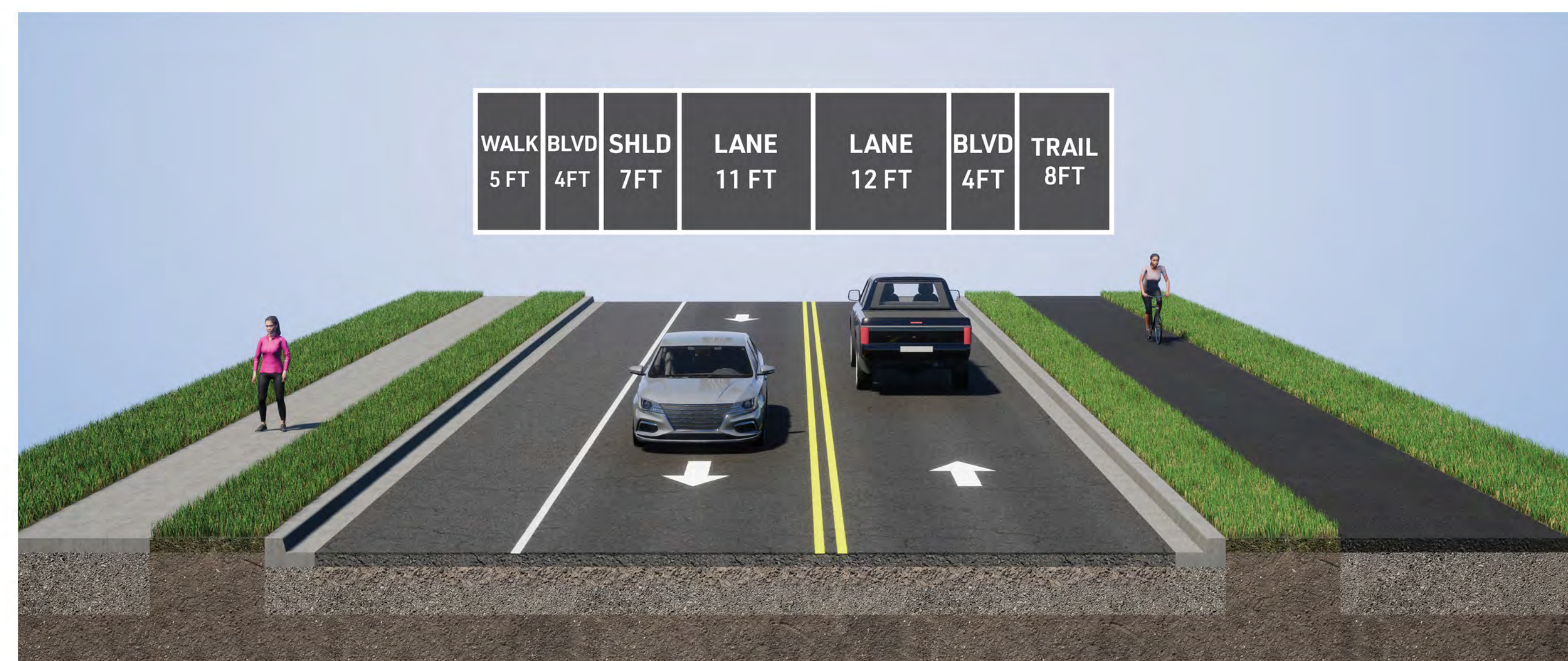
Proposed Butler Avenue Typical Section (Looking East)
