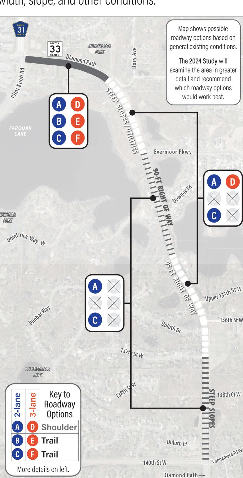
Roadway Options (Based on an average right-of-way width of 100 feet.)
