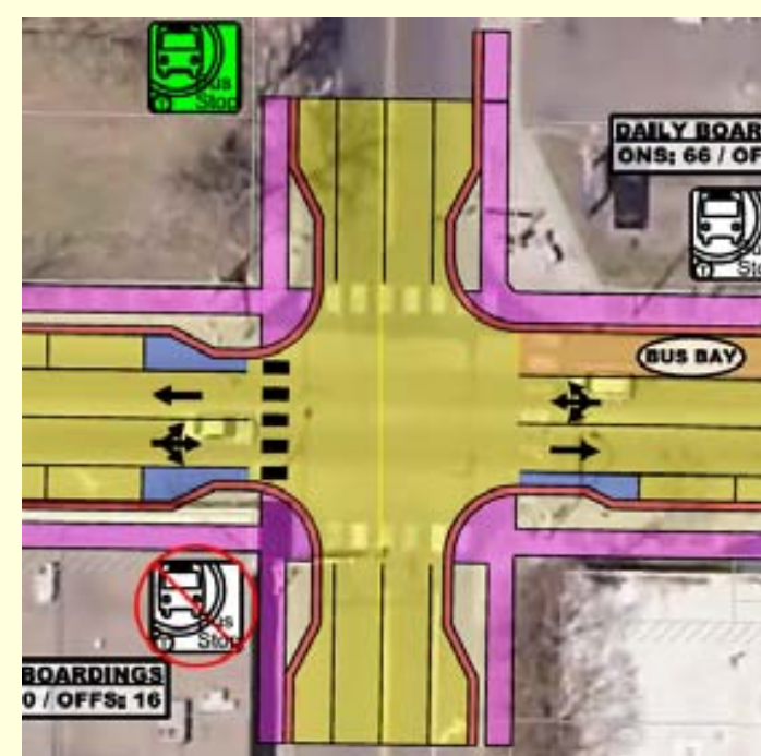
Thru-stop (side street stop) control is recommended
