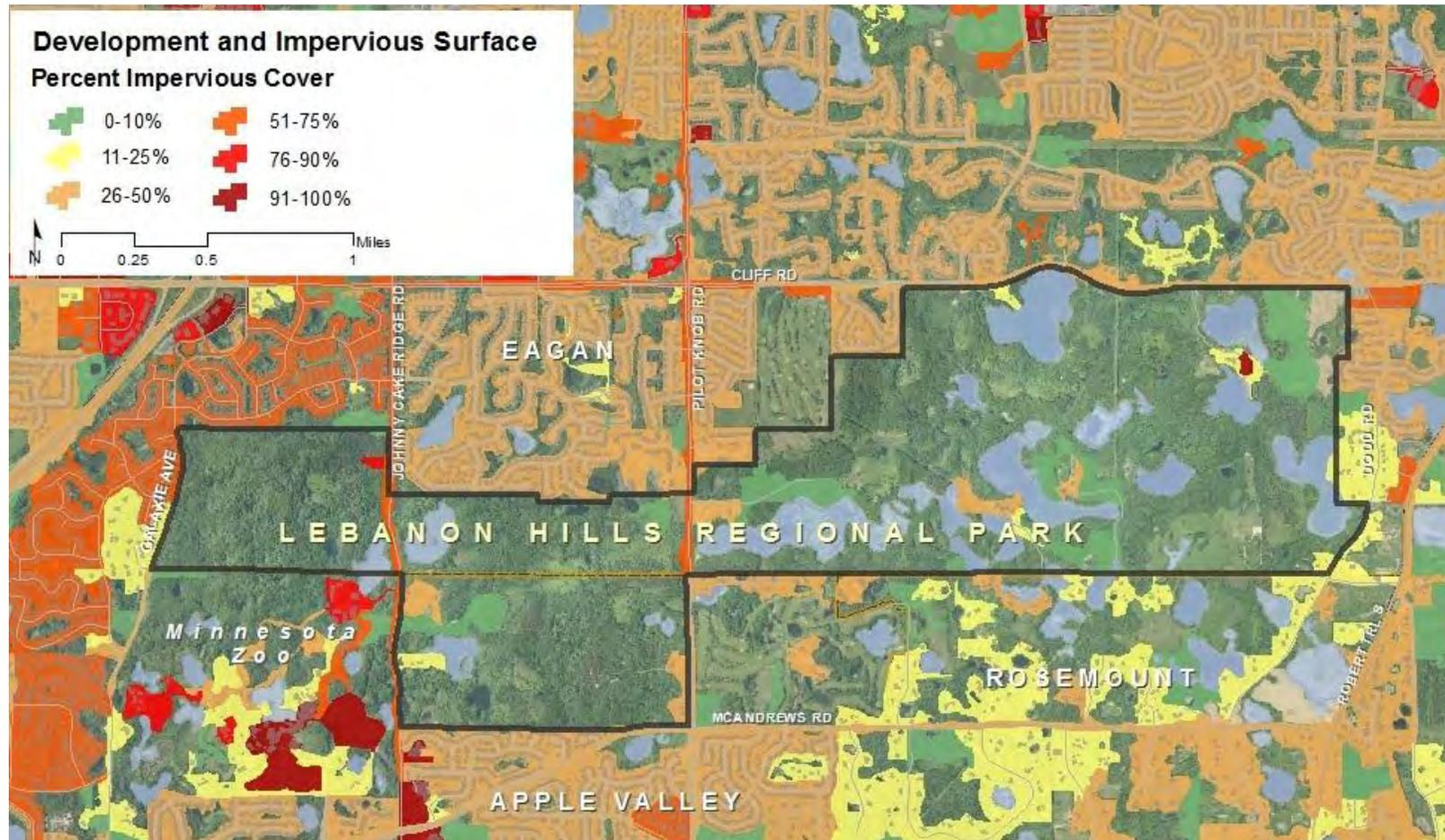
Increased stormwater flows entering the park have contributed to channel and bank erosion on the park's creeks and waterways. Lake and wetland bounce has killed shoreline vegetation and de-stabilized shoreline soils. Deposition of eroded materials has formed alluvial fans in park lakes and contributes to lake infilling.
