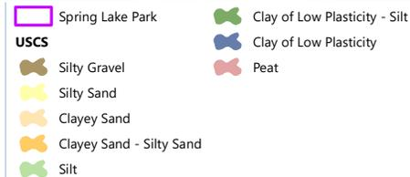
The Unified soil classification system (USCS) classifies mineral and organic mineral soils for engineering purposes on the basis of particle-size characteristics, liquid limit, and plasticity index.
