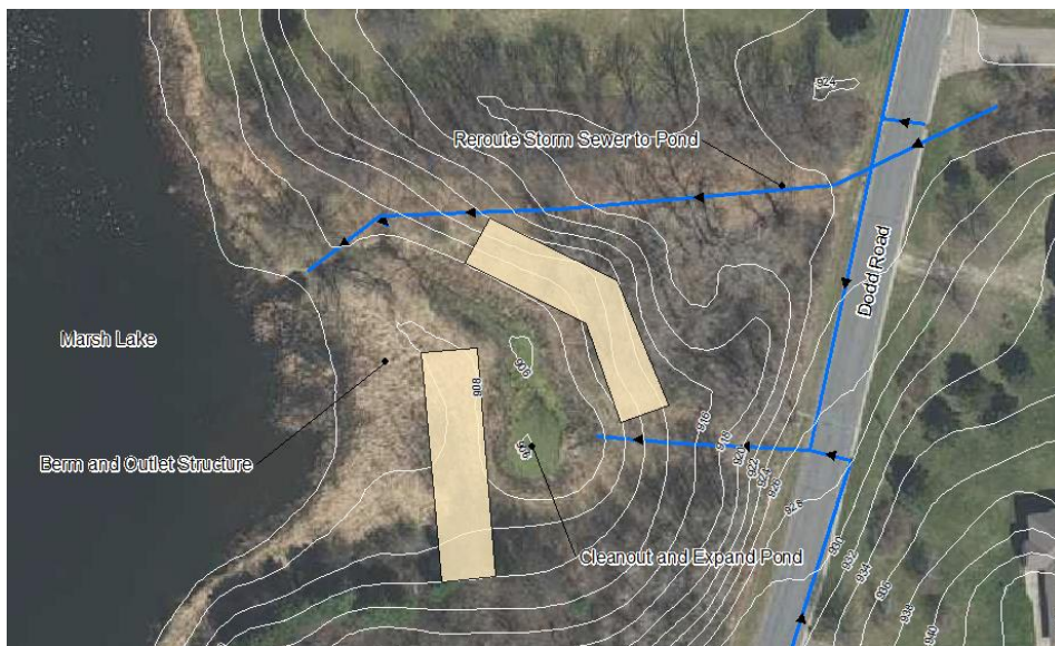
Concept overview of proposed filter bench locations (tan rectangle) and approximate sizes. Blue lines indicate existing storm sewer infrastructure.
