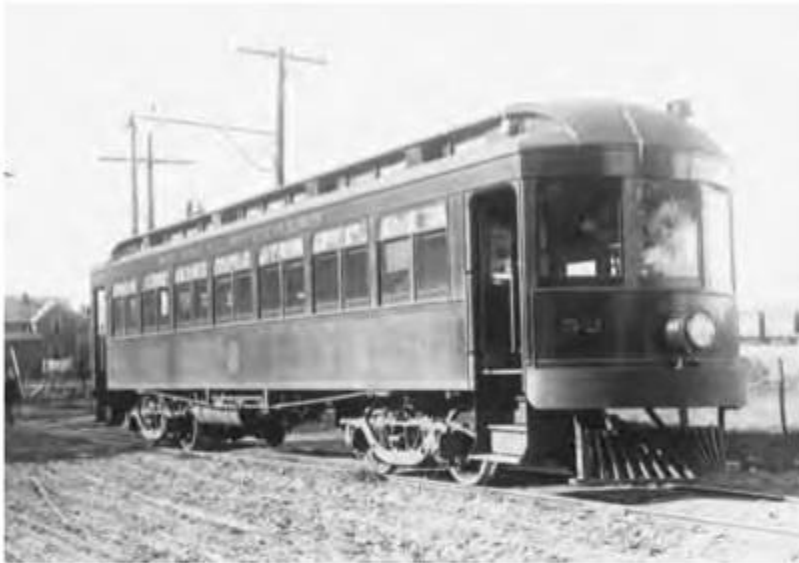
Car 52 was one of four interurbans built by the Niles Car Company of Niles, Ohio, at a cost of $8,490 and delivered to the Southern in 1914. The cars were all wood construction with a wood under-frame—unusual in that steel cars were coming into general use. Car 52 was 51 feet long and weighed 29 tons. It could accommodate 54 passengers—moving them along at a top speed of 55 miles per hour. This photo was taken in the Inver Grove yard sometime before 1920. Photo courtesy of the Minnesota Streetcar Museum.
