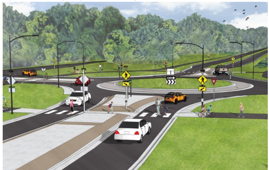
Figure 3-8: Example of RRFB at a Single-Lane Roundabout
