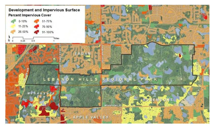
Increased stormwater flows entering the park have contributed to channel and bank erosion on the park's creeks and waterways. Lake and wetland bounce has killed shoreline vegetation and de-stabilized shoreline soils. Deposition of eroded materials has formed alluvial fans in park lakes and contributes to lake infilling.
